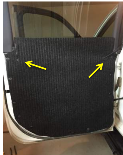
Figure 52: Door Cover Fabric Initial Placing
