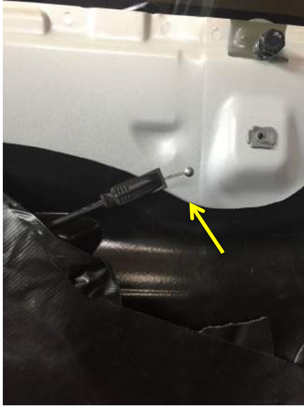
Figure 53: Original Door Cable
