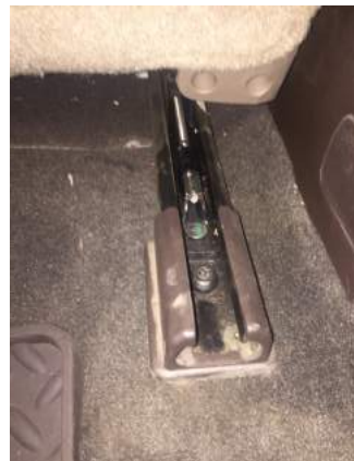
Figure 5: Star Bolt Removal 2
